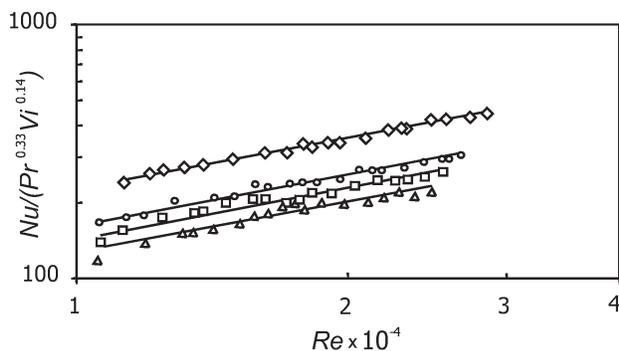
**Fig. 2.** The dependence  $Nu/(Pr^{0.33}Vi^{0.14}) = f(Re)$  for the baffled and unbaffled agitated vessel with the HE 3 impeller and constant  $H/D = 0.5$ : diamonds –  $J = 4$ ,  $e/R = 0$ ; squares –  $J = 0$ ,  $e/R = 0$ ; triangles –  $J = 0$ ,  $e/R = 0.27$ ; circles –  $J = 0$ ,  $e/R = 0.53$ .
