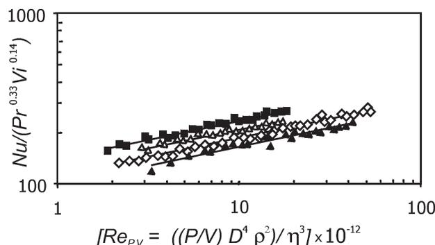
**Fig. 4.** The dependence  $Nu/(Pr^{0.33}Vi^{0.14}) = f(Re_{P,V})$  for the liquid aspect ratio  $H/D = 1$  and HE 3 impeller: diamonds –  $J = 4$ ,  $e/R = 0$ ; filled triangles –  $J = 0$ ,  $e/R = 0$ ; opened triangles –  $J = 0$ ,  $e/R = 0.4$ ; filled squares –  $J = 0$ ,  $e/R = 0.53$ .
