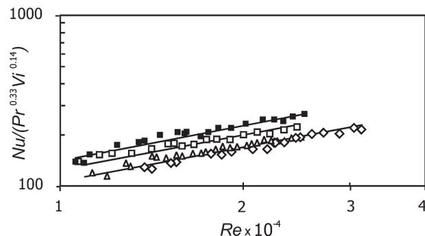
**Fig. 1.** The dependence  $Nu/(Pr^{0.33}Vi^{0.14}) = f(Re)$  for the unbaffled agitated vessel with the HE 3 impeller;  $H/D \neq \text{const}$ ;  $J = 0$ ; filled squares –  $e/R = 0$ ,  $H/D = 0.5$ ; squares –  $e/R = 0.13$ ,  $H/D = 0.5$ ; triangles –  $e/R = 0.13$ ,  $H/D = 1$ ; diamonds –  $e/R = 0.13$ ,  $H/D = 1.5$ .
