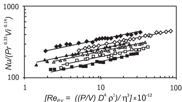
**Fig. 3.** The dependence  $Nu/(Pr^{0.33}Vi^{0.14}) = f(Re_{P,V})$  for the liquid aspect ratio  $H/D = 0.5$ : diamonds –  $J = 4$ ,  $e/R = 0$ ; squares –  $J = 0$ ,  $e/R = 0$ ; triangles –  $J = 0$ ,  $e/R = 0.53$ . Opened symbols – HE 3 impeller; full symbols – propeller agitator.
