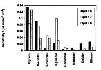
Fig. 2. Response of the *Gluconobacter* sp. membrane-based biosensor to various substrates. The sensitivity was measured in three buffer solutions: acetate, pH 6, phosphate, pH 7, and glycine, pH 8.
