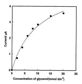
Fig. 1. Calibration graph of the glycerol biosensor in 0.05 mol  $dm^{-3}$  sodium acetate buffer (pH = 6).
