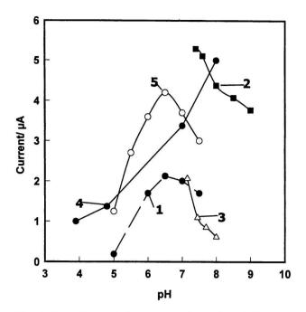
Fig. 3. Dependence of the response of the glycerol biosensor on pH in different buffer solutions. The glycerol concentration was 5 mmol  $dm^{-3}$  (1. phosphate buffer, 2. borate buffer, 3. tris-malate buffer, 4. glycine buffer, 5. acetate buffer).
