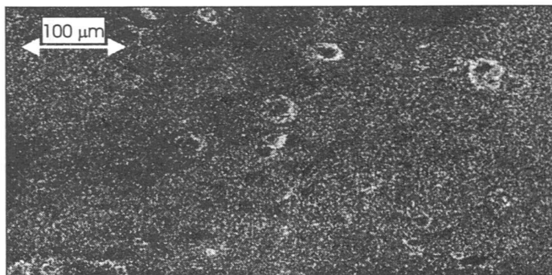
Fig. 6. Surface morphology of layers, thermal treatment at 800 °C for 4 h.
