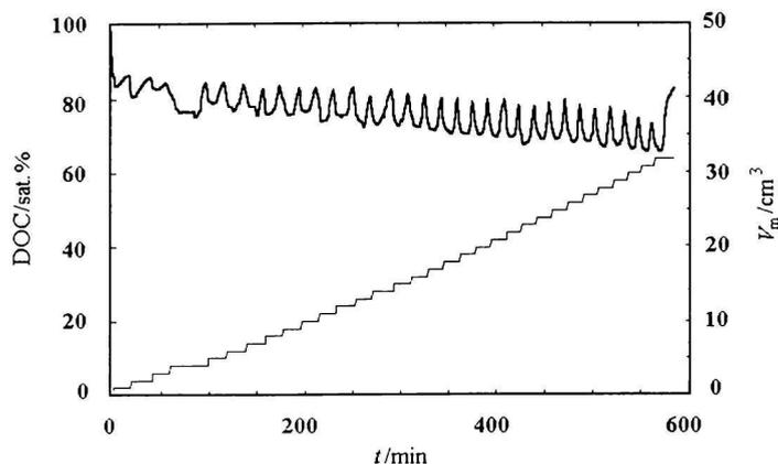
Fig. 2. Dissolved oxygen concentration as a controlled variable: time dependence of cultivation medium volume added into the bioreactor and the course of the controlled variable concentration. DOC – dissolved oxygen concentration (saturation %) (—),  $V_m$  as in Fig. 1.
