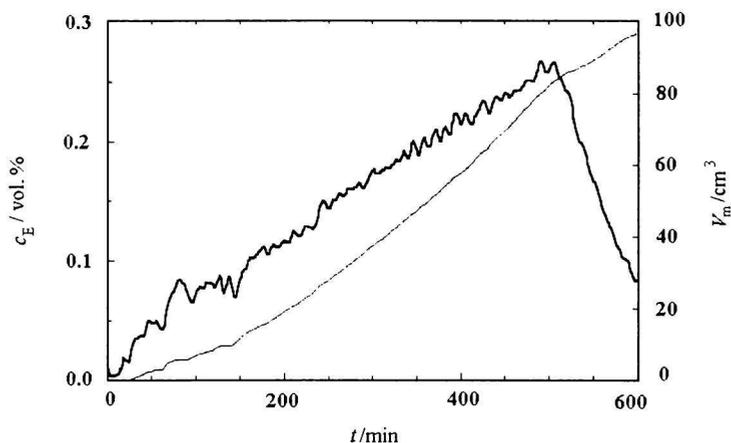
Fig. 4. Ethanol concentration as a controlled variable: time dependence of cultivation medium volume added into the bioreactor and the course of the controlled variable concentration.  $c_E$  as in Fig. 3,  $V_m$  as in Fig. 1.
