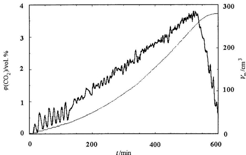
Fig. 1. Carbon dioxide concentration as a controlled variable: time dependence of cultivation medium volume added into the bioreactor and the course of the controlled variable concentration.  $V_m$  – total volume of the medium A ( $\text{cm}^3$ ) fed into the bioreactor (—),  $\varphi(\text{CO}_2)$  – vol. % of  $\text{CO}_2$  in gas phase (---).
