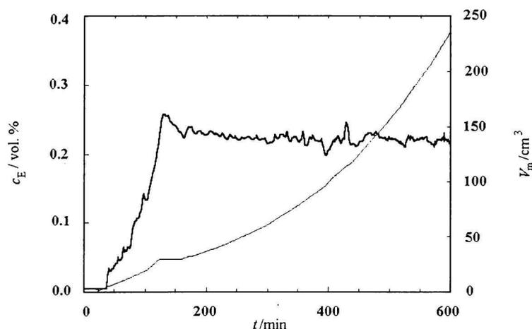
Fig. 3. Ethanol concentration as a controlled variable: time dependence of cultivation medium volume added into the bioreactor and the course of the controlled variable concentration.  $c_E$  – ethanol concentration in cultivation medium (vol. %) (—),  $V_m$  as in Fig. 1.
