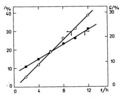
Fig. 1. Dependence of conversion (C) and grafting efficiency (G) of vinyl chloride on polymerization time using the  $Fe^{2+}$ —Chelaton 3 system.
