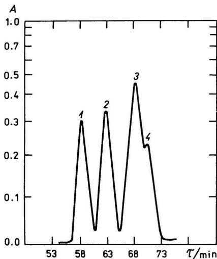
Fig. 3. Record of the separation of lanthionine and selenolanthionine on a 62 cm long catex column eluted with a pH 3.25 buffer.
