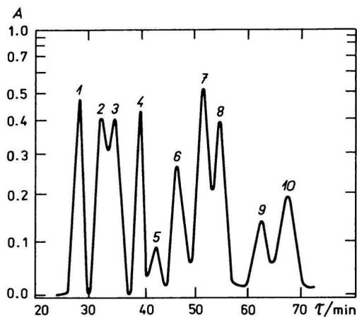
Fig. 1. Separation of a standard mixture of amino acids containing selenolanthionine on a catex column (37 × 0.8 cm) eluted with a pH 3.25 buffer.
