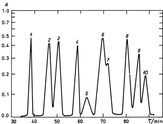
Fig. 2. Separation of a standard mixture of amino acids containing selenolanthionine in a catex column (62 × 0.8 cm) eluted with a pH 3.25 buffer.
