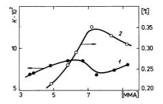
Fig. 2. Dependence of the ratio K (from Table 1) (curve 1) and of the limiting viscosity number  $[\eta]$  in  $[dl g^{-1}]$  (curve 2) of poly(methyl methacrylate) having number average molecular weight  $M_n = 6.1 \times 10^4$  in the mixture MMA—methanol on molar concentration of methyl methacrylate; temperature 30°C.
