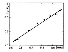
Fig. 1. Dependence of the log of MMA polymerization rate [mol dm<sup>-3</sup> s<sup>-1</sup>] on the log of MMA concentration [mol dm<sup>-3</sup>] in methanol. Concentration of AIBN  $5 \times 10^{-3}$  mol dm<sup>-3</sup>; in-
