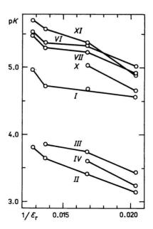
Fig. 1. pK Value of amide oximes as a function of reciprocal value of relative permittivity of the solvent.
