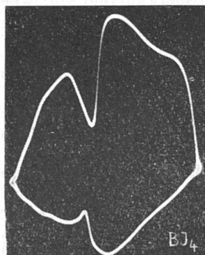
Fig. 4. Curve dE/dt = f(E) of dextransulphate B_{13} , conc. 1 mg/ml in 1 M citric acid medium.
