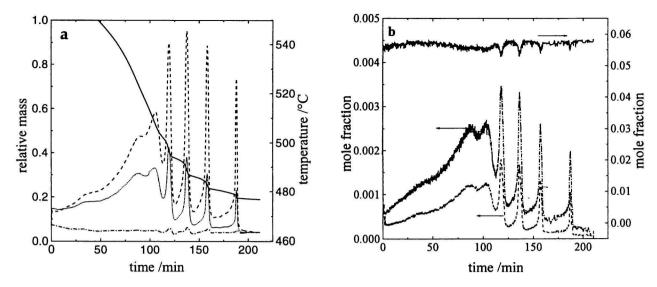
Fig. 3. Combustion of coal char particle at 460 °C and 5 mole % oxygen content. a) Time dependences of the mass of particle (solid line), temperature in the centre of the particle (dashed line), temperature on the geometrical surface (dotted line), temperature of the gas phase close to the particle surface (dot-dashed line); b) Flue gas composition vs. time. Oxygen - solid line, carbon dioxide - dashed line, carbon monoxide - dot-dashed line.
