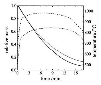
Fig. 1. Combustion of coal char particle at different initial temperatures and 15 mole % feed oxygen content. The mass of particle and temperature in the centre of the particle vs. time; 527 °C: solid line and dot-dashed line, respectively; 627 °C: dotted and dashed line, respectively.
