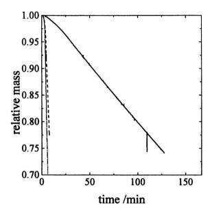
Fig. 2. Combustion of coal char particle at a low temperature (460 °C) and different oxygen contents. The mass of particle vs. time dependences. Solid line - 5 mole %, dashed line - 10 mole %, dotted line - 15 mole %.
