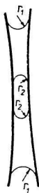
Fig. 2a. Tubular tapered pore: r_1 — equilibrium radius of meniscus of condensed phase; r_2 — radius of nucleus; r_1 > r_2 .
